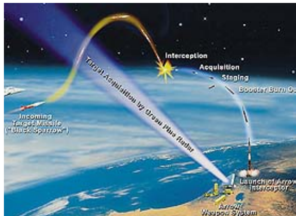
Graphic illustrates how the Arrow 2 intercepted a Black Sparrow target missile fired from a Boeing F-15 fighter. (Source: IAI)
